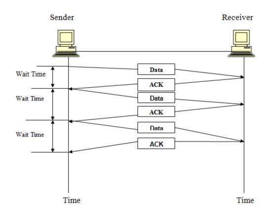
The advantage of stop and wait is simplicity: each frame is checked and acknowledged before the next frame is sent. The disadvantage is inefficiency: stop and wait is slow. Each frame is alone on the line. If the distance between devices is long, the time spent waiting for ACKs between each frame can add significantly to the total transmission time.
